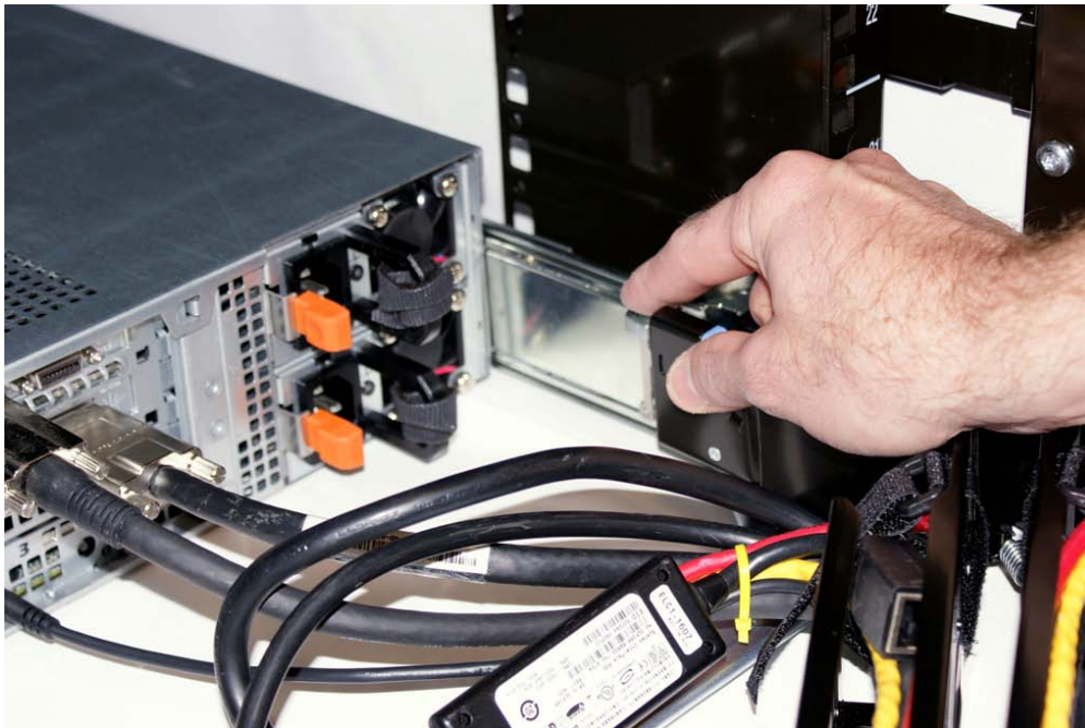
Figure 9: Disconnecting the Inner CMA Attachment Bracket
